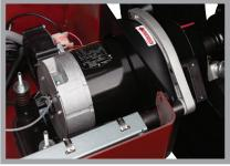
The motor and spindle are combined into a single, pre-balanced assembly that always stays calibrated to zero.
