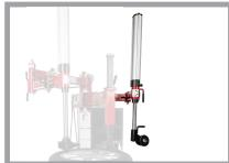
The RoboRoller<sup>™</sup> provides additional power when mounting difficult tire assemblies by preventing the bead from rolling back over the mount tool.
