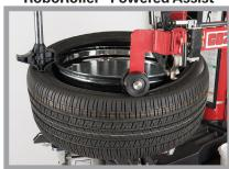
The RoboRoller® provides additional power when mounting difficult tire assemblies by preventing the bead from rolling back over the mount tool.
